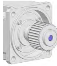
5. Screw the washer using the hexagon socket screw onto the drive pin.
