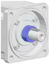
2. Push on the spacer washer above the key on the drive pin until it touches the base.
